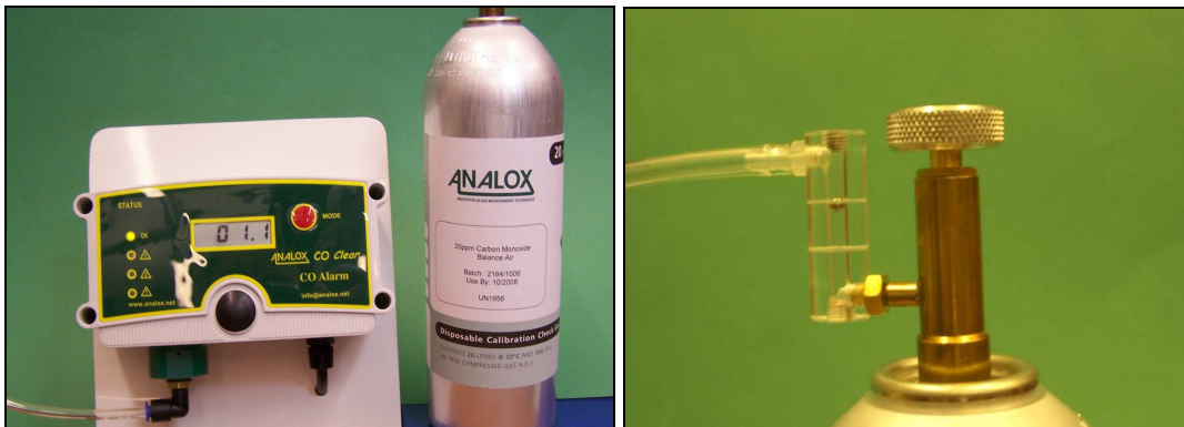
Connecting of the gas cylinder
